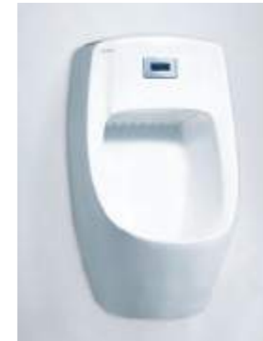
Sensor urinoir Integral battery operated, infrared sensor operated flush with pre flush 250 ml, post flush 350 ml and concealed water inlet Q357610110 MRP. ₹ 25,175
