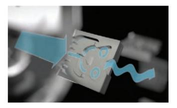
Each channel is designed to create a vortex that oscillates water and sculpts it as it exits into a wave pattern that provides a dense, concentrated spray—to give the feeling of an indulgent shower, without wasting water.
