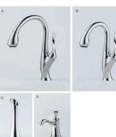
A. SINGLE-HANDLE PULL-DOWN 63052LF-PC Height: 15" Reach: 91/2" Max Flow: 1.8 gpm @ 60 psi
