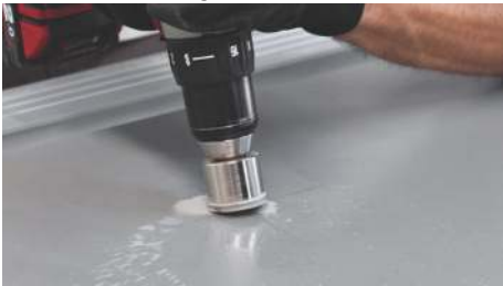
1. Round Cut with Diamond Blade Drill
